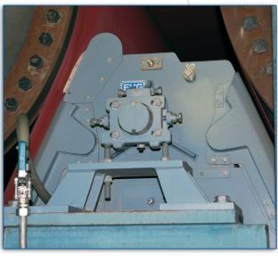
With the EV EasyOne it is possible to improve the web release effectively with a special high vacuum area. This optimizes both drying section runnability and draws to improve paper quality.
